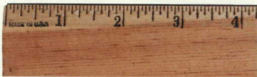
a. Common ruler where the 0 (starting point) is implicit at the edge
